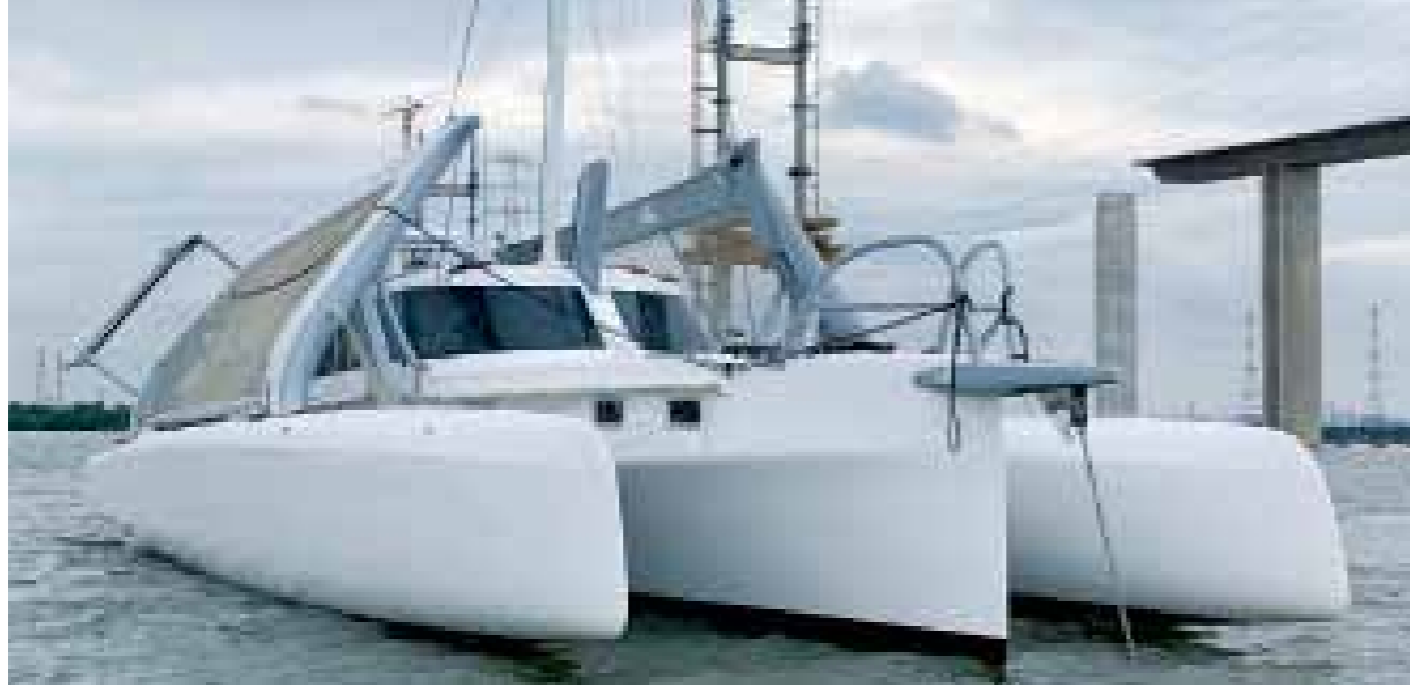
ABOVE: Sea trials in Vietnam of the Rapido 50's folding amas (with a demonstration mast installed). Image Rapido
